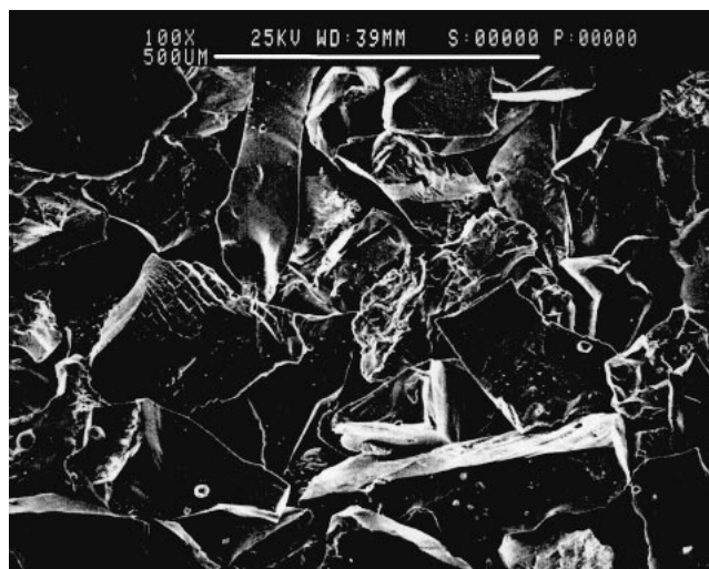
Fig. 2 Scanning electron micrograph of alumina particles
